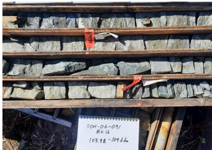
Figure 2-1 Mineralised intersection from drillhole 06-91. Note that the wooden core blocks and sample tags are still legible. (D. James June 2025)
