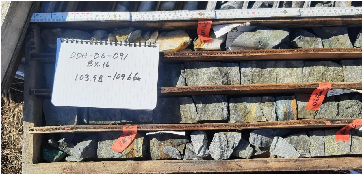
Figure 10-2 Example interval of sulphide core from drillhole 06-091 showing the good condition of the core (June 20, 2025)
