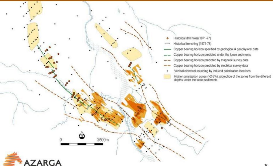
Historical plan view and selected cross-sections indicate a syncline of copper-bearing ore
